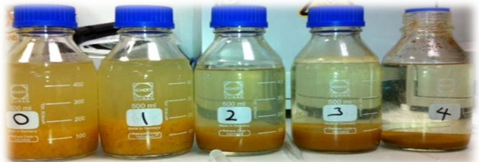
Oil Platform Wastewater Treated with Electrocoagulation
